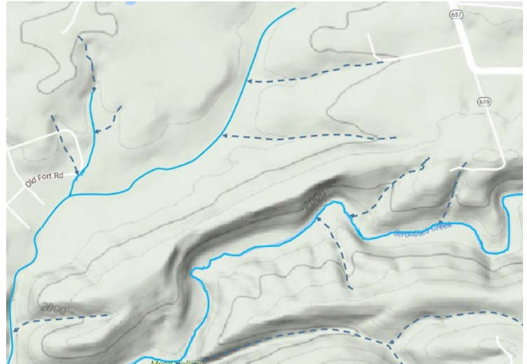
Figure 14. Drainageways are sloping waterways (blue dashed arrows) that carry water to more level flood plains (solid blue line). Drainageways in cropland may have perennial grass planted to prevent erosion (grassed waterways). Terrain view (Map Data 2017 Google). Annotated by John M. Galbraith, Virginia Tech.
