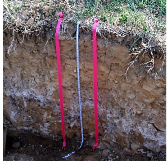
Figure 16. Fragipans (dense horizon below the white colors) have slow permeability, forming a water perching zone. Some have dominantly white colors. Photograph courtesy of Erik Severson, Virginia Tech.
