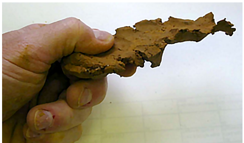
Figure 5: Guide to estimating one of 12 texture classes by hand from a moist, mixed soil sample about the size of an egg. This sample makes a ribbon over 4 inches long and is not very gritty, and would be classified as a clay, or silty clay, depending on how much grit could be felt. Photo courtesy of John Galbraith, Virginia Tech.
