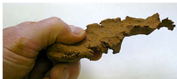
Figure 5: Guide to estimating one of 12 texture classes by hand from a moist, mixed soil sample about the size of a ping-pong ball. This sample makes a ribbon over 2 inches long so it would be classified in the clay family. Photo courtesy of John Galbraith, Virginia Tech.
