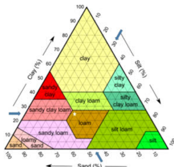
Figure 4: The texture triangle relates the percent sand, silt and clay to one of 12 texture classes. Thick arrows show the direction to read the values. A soil with 25% clay, 45% sand, and 30% silt (white star) would be a “loam” texture. Soil. (Reprinted from https://en.wikipedia.org/wiki/Soil ). Drawn by Mike Norton, redrawn from USDA-NRCS Soils web page ( https://www.nrcs.usda.gov/wps/portal/nrcs/site/soils/home/ ).
