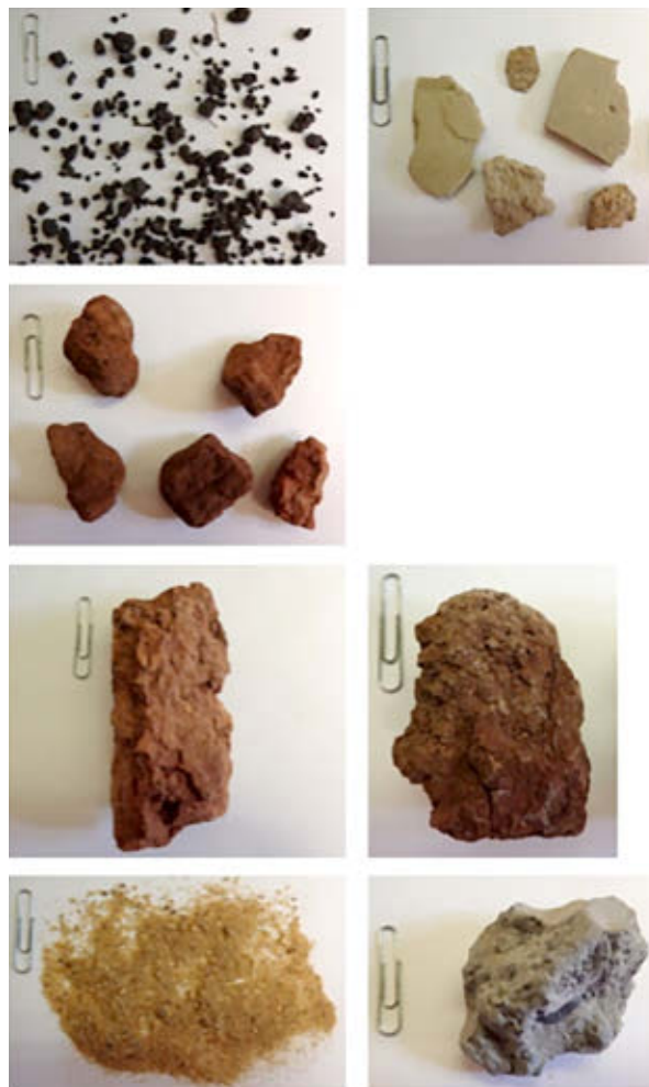
Figure 9. Several shapes of soil structure. Listed left to right, top row to bottom row: granular, platy, and blocky; prismatic and columnar; structureless coherence of single grained and massive shape. Photos copyright, courtesy of John M. Galbraith, Virginia Tech.
