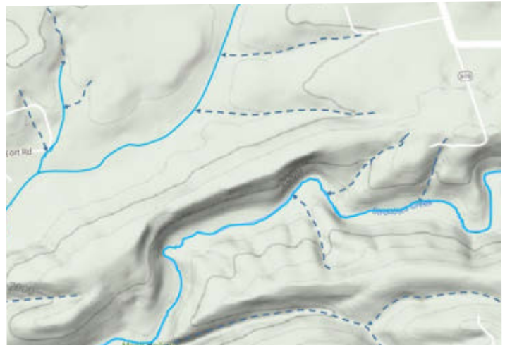
Figure 14. Drainageways are sloping ephemeral streams (blue dashed arrows) that carry water to more level flood plains (solid blue line). Drainageways in cropland may have perennial grass planted to prevent erosion (grassed waterways). Terrain view (Map Data 2017 Google). Annotated by John M. Galbraith, Virginia Tech.
