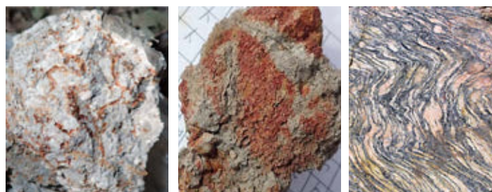
Figure 8. Left: red wetness mottles (redoximorphic features) in a gray colored horizon. Photo from U.S. Department of Agriculture. Center: gray wetness mottles (redoximorphic features) in a red colored horizon. Right: consistent, parallel, linear color patterns in bedrock leaves behind lithochromic color patterns as the rock weathers into soil. Soil photos courtesy Ben Smith and John M. Galbraith, Virginia Tech. Gneiss. accessed 3-15-2017, By Huhulenik - Own work, CC BY 3.0, https://commons.wikimedia.org/w/index.php?curid=15036586
