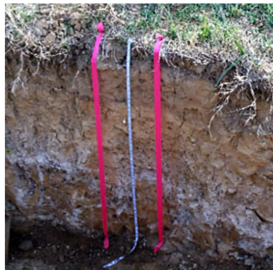
Figure 15. Fragipans (dense horizon below the white colors) have slow permeability, forming a water perching zone. Photograph courtesy of Erik Severson, Virginia Tech.
